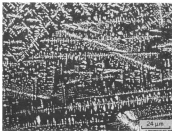
Figure 2 The microstructure of A-S13 alloy as chill-cast. 8.2 cm wide × 6.2 cm deep.
