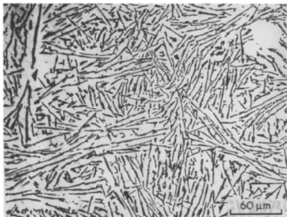
Figure 1 The microstructure of high purity sand-cast eutectic alloy. 7.6 cm wide × 5.8 cm deep.
